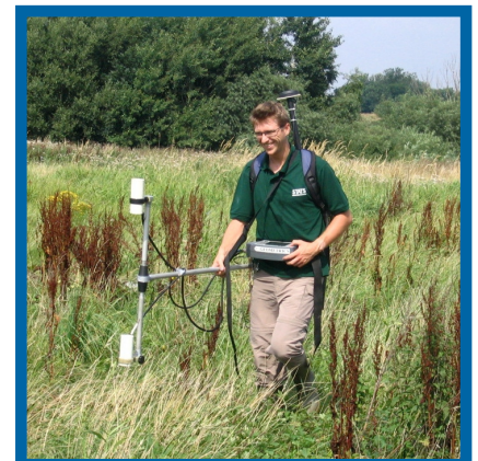
Surface mapping for UXO using magnetometry
